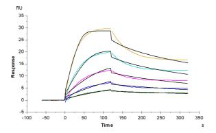
Mouse FcRn, His Tag captured on CM5 Chip via anti-his antibody can bind Trastuzumab with an affinity constant of 1.76 nM as determined in SPR assay (Biacore T200) (QC Test).
