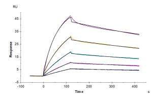
Mouse FcRn, His Tag captured on CM5 Chip via anti-his antibody can bind Mouse IgG1 Fc, No Tag with an affinity constant of 15.09 nM as determined in SPR assay (Biacore T200).
