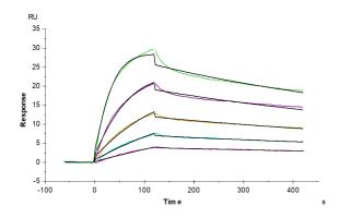
Mouse FcRn, His Tag captured on CM5 Chip via Anti-His Antibody can bind Mouse IgG2a Fc, No Tag with an affinity constant of 2.72 nM as determined in SPR assay (Biacore T200).
